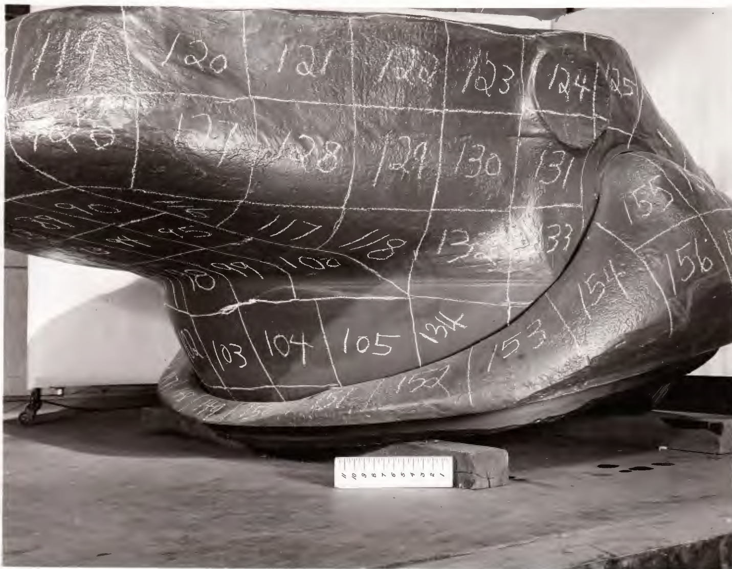
A88724 CONFIDENTIAL 8 ABERDEEN PROVING GROUND 8 20 April 1953 Project No. TT2-586. Tank, Turret, Oscillating, Serial No. 3. Three-quarter right rear view showing thickness measurement locations before test at APG.
