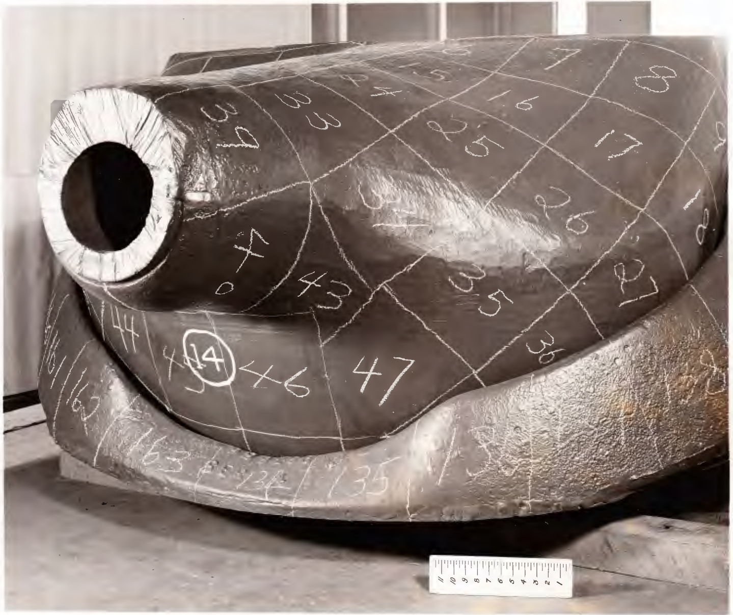
A88722 CONFIDENTIAL ABERDEEN PROVING GROUND 20 April 1953 Project No. TT2-586. Tank, Turret, Oscillating, Serial No. 3. Three-quarter left front view showing thickness measurement locations before test at APG.
