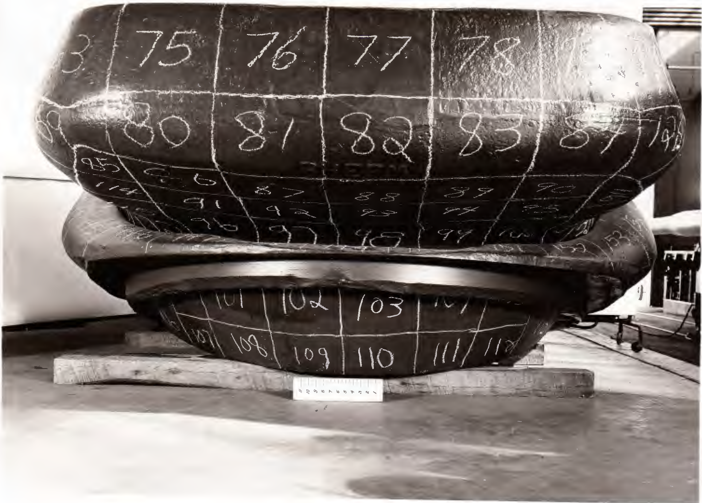
A88719 CONFIDENTIAL Ⓢ ABERDEEN PROVING GROUND Ⓢ 20 April 1953 Project No. TT2-586. Tank, Turret, Oscillating, Serial No. 3. Rear view showing thickness measurement locations before test at APG.
