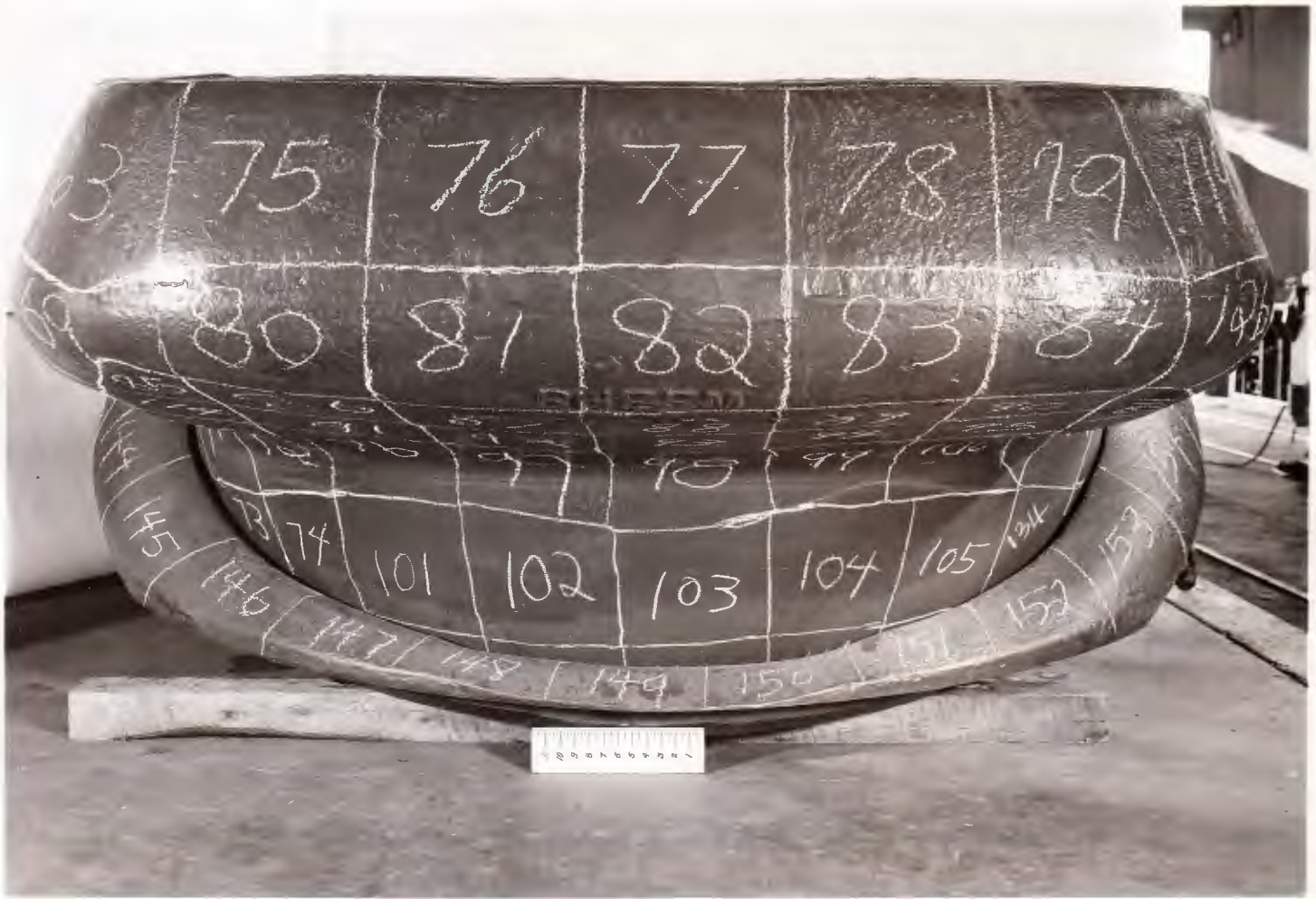
A88718 CONFIDENTIAL 8 ABERDEEN PROVING GROUND 8 20 April 1953 Project No. TT2-586. Tank, Turret, Oscillating, Serial No. 3. Rear view showing thickness measurement locations before test at APG.
