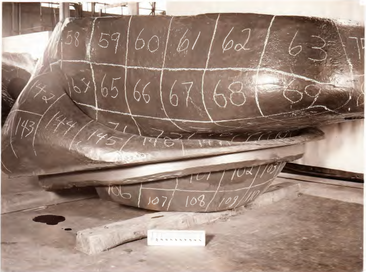
A88726 CONFIDENTIAL § ABERDEEN PROVING GROUND § 20 April 1953 Project No. TT2-586. Tank, Turret, Oscillating, Serial No. 3. Three-quarter left rear view showing thickness measurement locations before test at APG.
